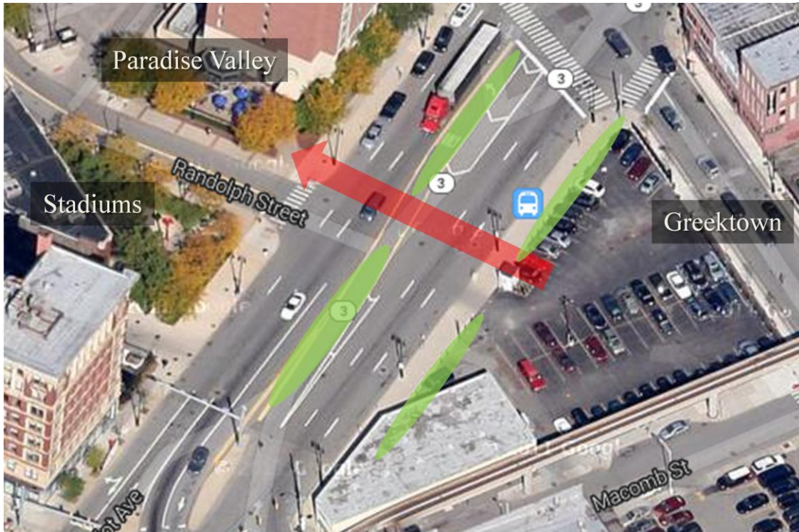
Example of median and parking lot landscaping to potentially deter jaywalking and give pedestrians refuge at preferred crossing locations. (Source: Google Maps)
